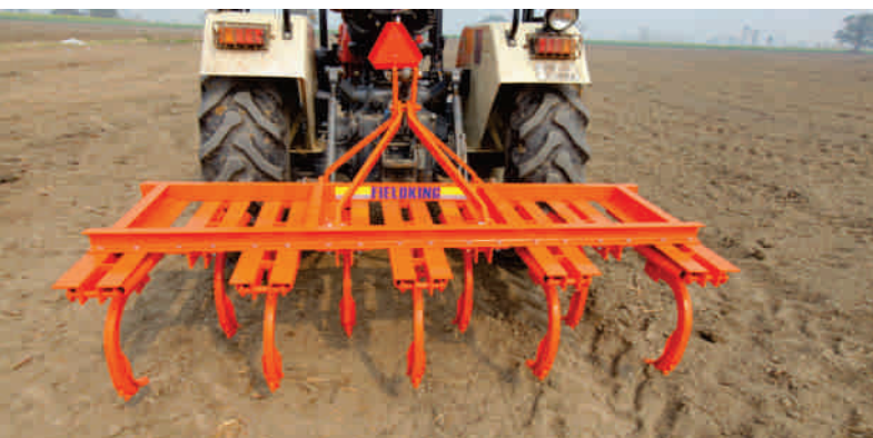
Spring having more capacity of absorbing shock
